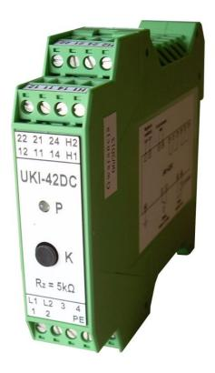
Control relay insulation UKI-42DC is a relay for monitoring the value of earth insulation resistance in isolated DC grids with a rated voltage range from 24V to 42VDC. The relay is designed for use on the ground or underground mining excavations of non-hazardous methane and class A coal dust explosion hazard.
